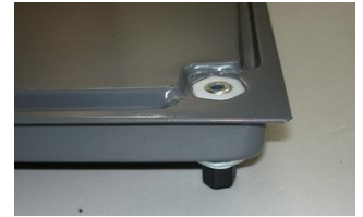
Socket-Set-Crew fixed inside and at top of pedestal
